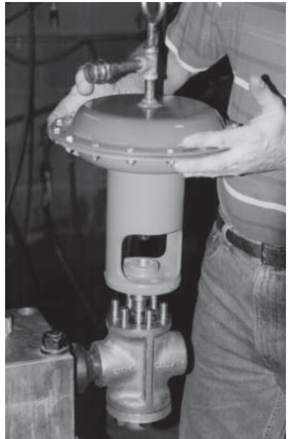
REMOVE HOUSING TO EXPOSE PACKER
