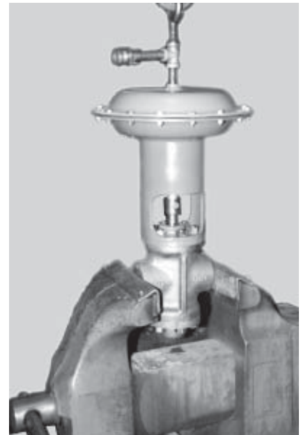
PROPER MOUNTING IN A VISE
