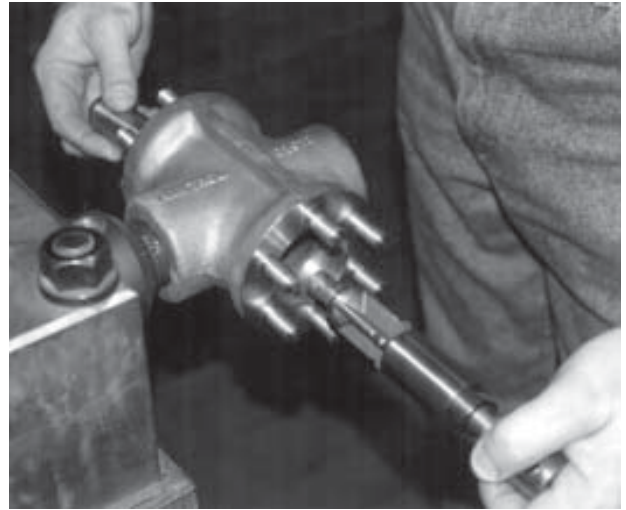
INSERT DISC PISTON AND SCREW TOGETHER
