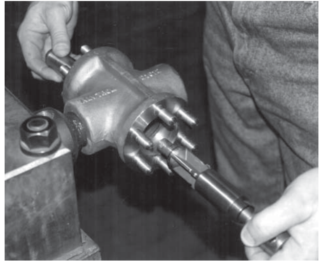
INSERT DISC AND PISTON AND SCREW TOGETHER
