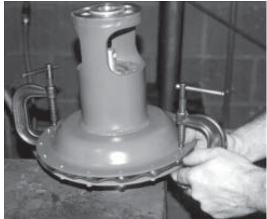
C-CLAMPS HELP DRAW DOWN THE HOUSING
