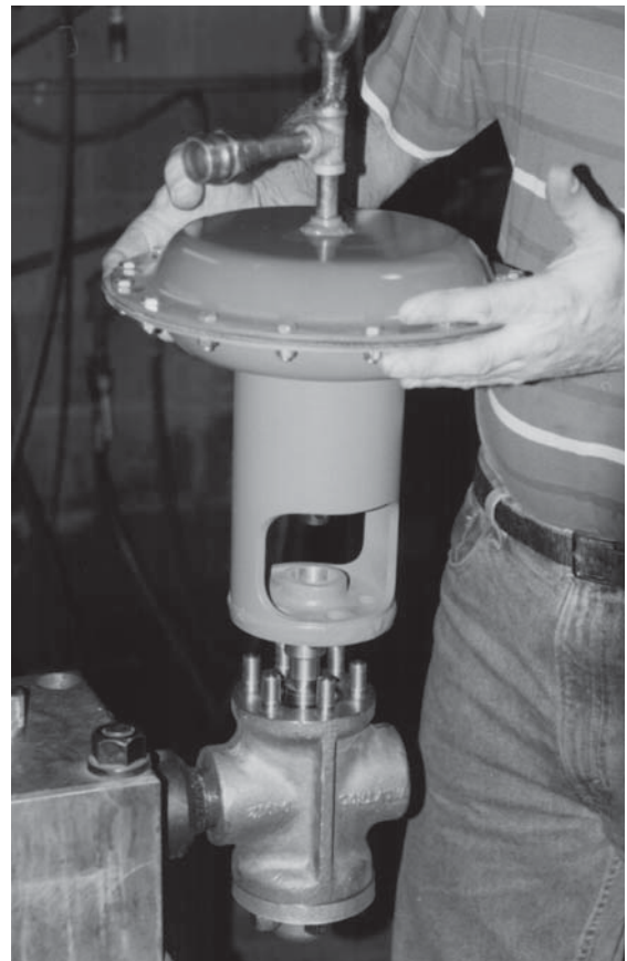
REMOVE HOUSING TO EXPOSE PACKER
